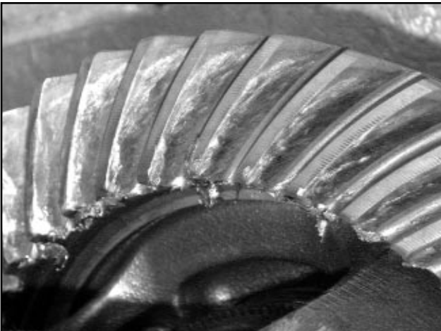
Burned ring & pinion
