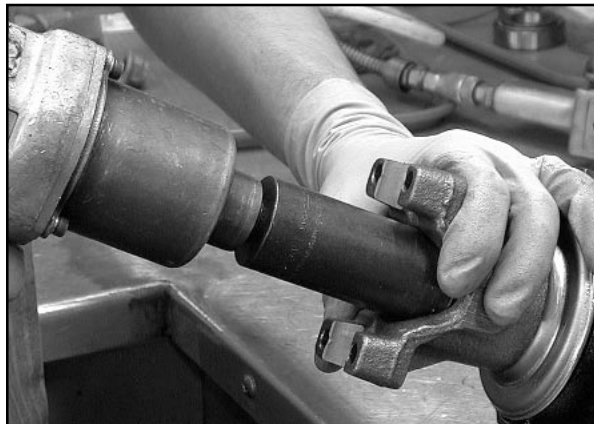
Impact on pinion nut
